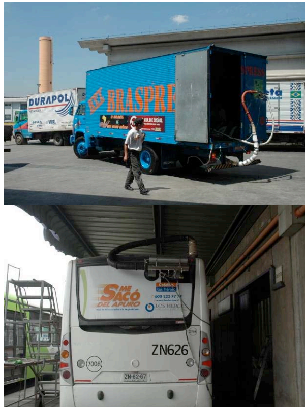
Figure 1: Truck and Bus with Flow Measurement Devices Connected to the Exhaust
