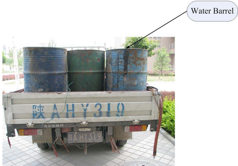
Figure 3: Exterior of a Truck Outfitted for Emissions Testing
