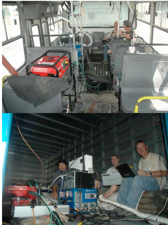
Figure 2: A Bus and Truck with Equipment and Sandbags Loaded
