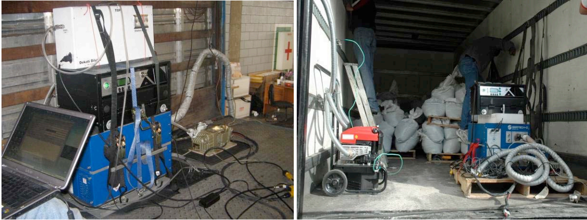
Figure 3b: Interior of Trucks Outfitted for Emissions Testing
