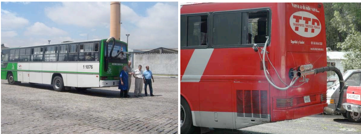
Figure 3a: Exterior of Buses Outfitted for Emissions Testing
