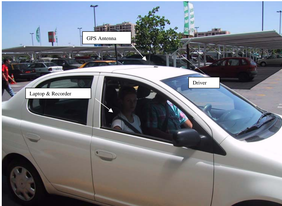
Figure III.1: GPS Instrumented Vehicle in Santiago, Chile
