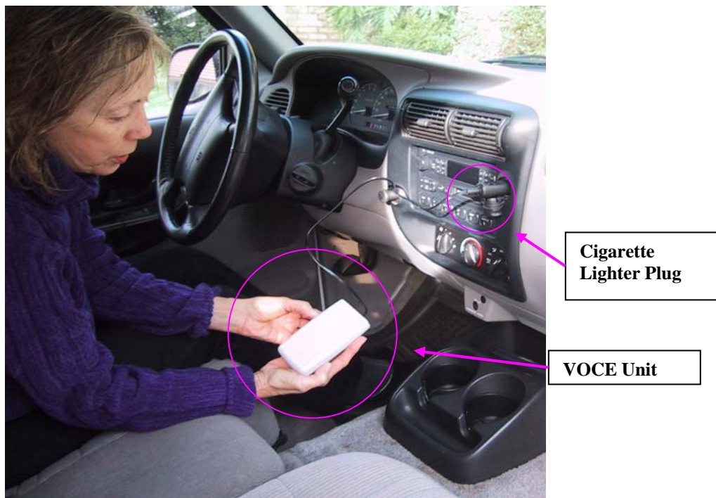
Figure A.7: VOCE Unit for Collecting Vehicle Start Information
