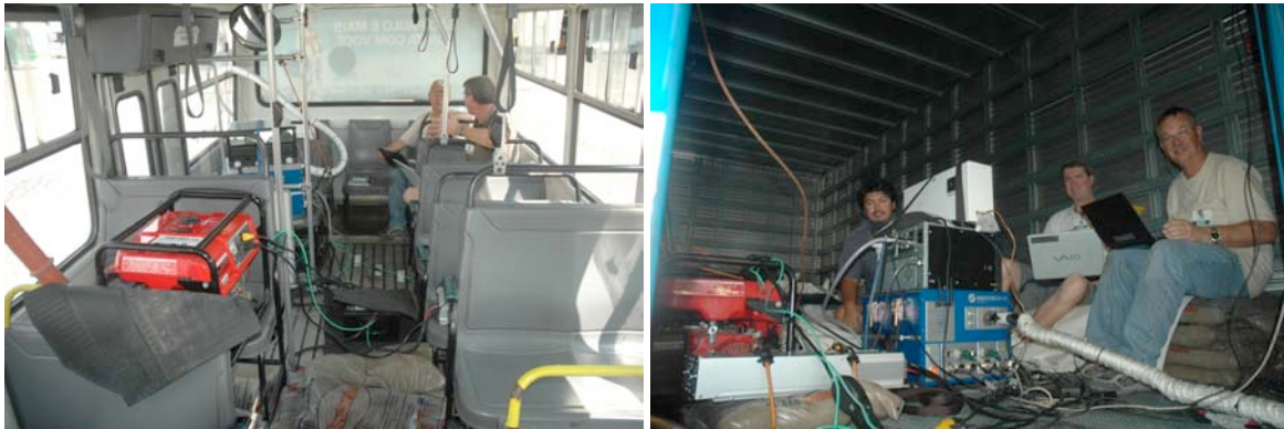
Figure 2: A Bus and Truck with Equipment and Sandbags Loaded
