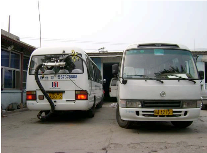
Figure 3: Exterior of Bus Outfitted for Emissions Testing
