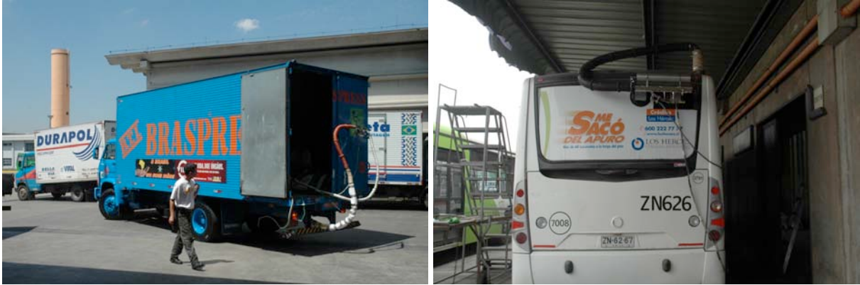
Figure 1: Truck and Bus with Flow Measurement Devices Connected to the Exhaust
