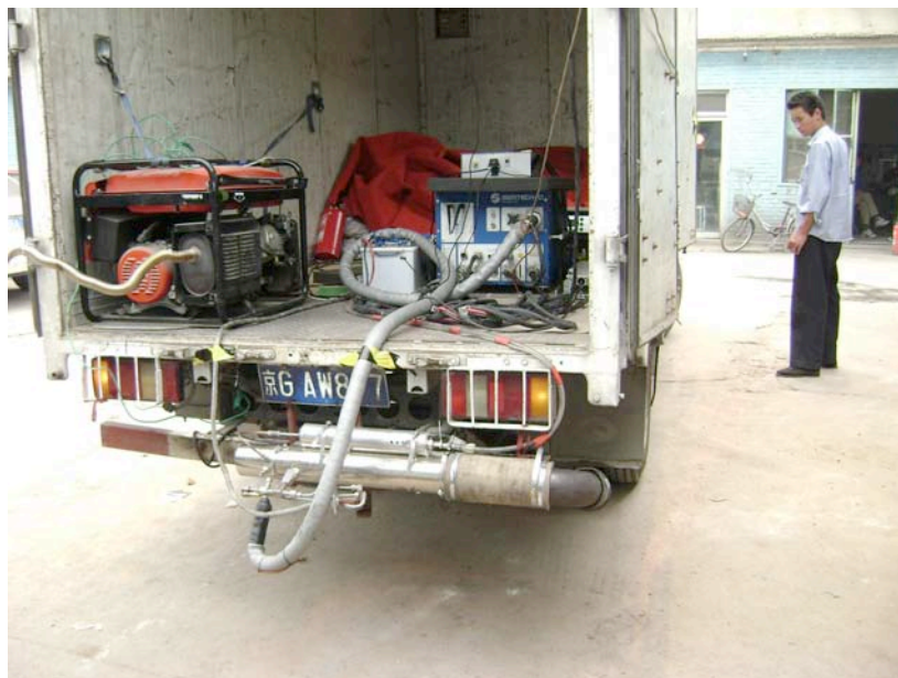
Figure 4: Exterior of a Truck Outfitted for Emissions Testing
