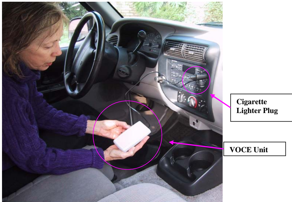
Figure VI.1 VOCE Unit for Collecting Vehicle Start Information
