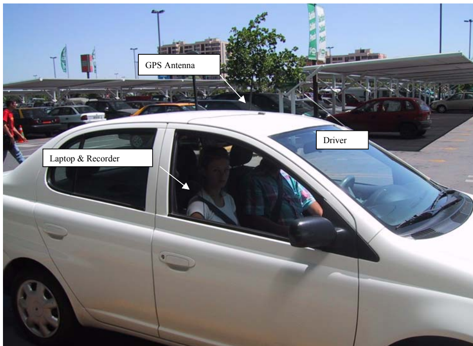
Figure III.1: GPS Instrumented Vehicle in Santiago, Chile
